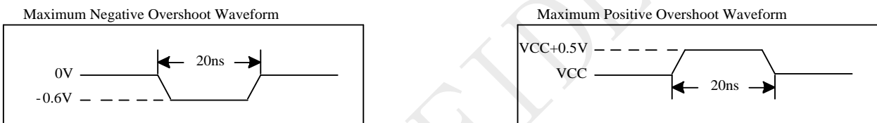
Figure 5-1 Maximum Overshoot Waveform
